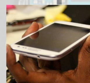
**7. Final examination:** The technician examines the exterior looking for issues with the glass or adhesive. The technician also examines the other functions such as the key board, camera, and power button.
