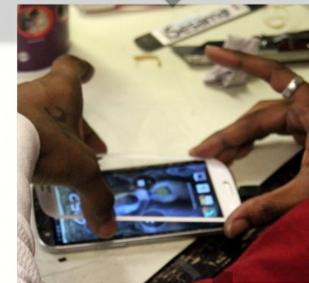
**6. Installation of the New Part:** The technician sets the new glass on top of the phone. Then presses and rubs fingertips along the edges assuring a smooth seal.
