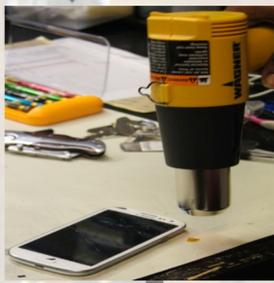
**2. Heating up of Broken Glass:** Technician waves a heat gun over the glass, warming the adhesive behind the glass. Technician repeatedly feels and checks the temperature to avoid damaging the LCD.
