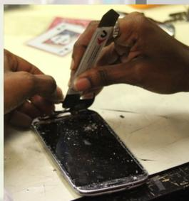
**3. Removal of Broken Part:** The technician moves between the heat gun and several specialized tools, working to carefully remove the broken glass.
