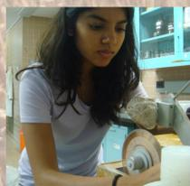
Figure 4: Sectioning valves using the diamond saw
